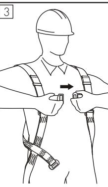
Connect chest strap buckle and adjust the tension the chest strap.
